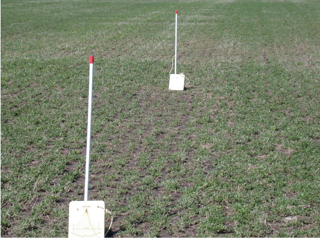
Stakes with slope finders to determine the slope for a land area.
