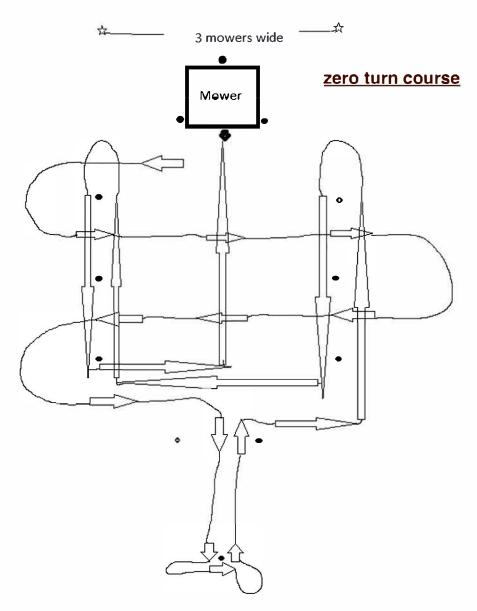
Mower Deck is no more than 3" from any post...when the mower passes through 2 posts they should be 6" wider than the mower deck. (i.e. mower deck = 48" posts will be 54" apart
